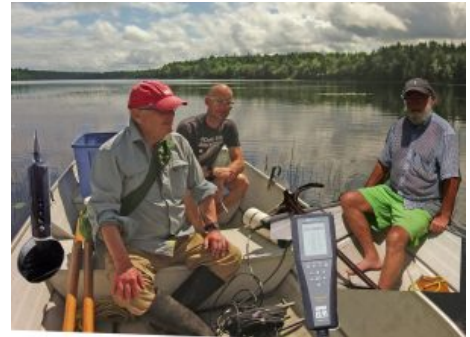
Water sampling on Sandy Lake, Aug 14, 2023 , here by the outlet. Insets: At left the YSI Probe with weight attached; right: YSI Instrument panel. A portion of the Van Dorn water sampling bottle can be seen by the anchor.
