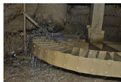
Figure 4: The water wheel (1) and the nozzle (2)
