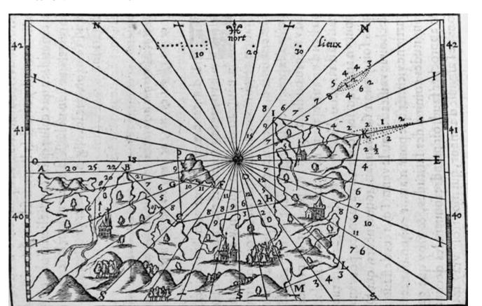
FIG. 51.5. CHAMPLAIN'S CHART TO ILLUSTRATE A COASTAL SURVEY. The lines A–B, B–C, C–H, etc., are successive legs of a survey along a hypothetical coast. The distances along each leg are carefully estimated and their bearing taken with a compass. Depth soundings are taken along each leg and important shoals. An example of triangulation is given for the leg B–C where sightings were taken to D, G, and F from B and C. A bar scale at ten-league intervals is given at the
